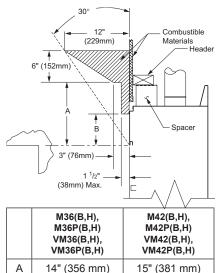
Figure 5 - Mantel Clearances - Side View (Cross Section)
